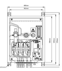
The nickel-plated brass bulkhead connections are suitable for 1/4" NPT and BSP male fittings & tubing. Internal components are brass, plastic fittings and tubing.
