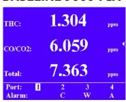
The 9000 Total Carbon analyzer utilizes a flame ionization detector (FID) in conjunction with a catalytic methanizer that converts the CO and CO2 to methane (CH4) and leaves the hydrocarbons unchanged for a total carbon measurement which is then subtracted from the total carbon concentration to determine the combined CO/CO2 reading.
